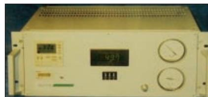
Figure 2 - VOC Canister Control module
